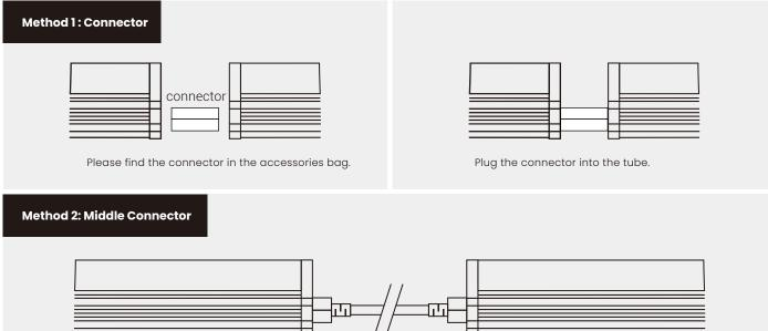
Please find the middle connector, Plug the middle connector into the tube.
