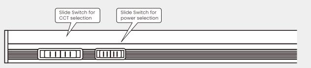
For the product with Slide Switch of wattage or CCT selection, please select the wattage or CCT needed before installation.
